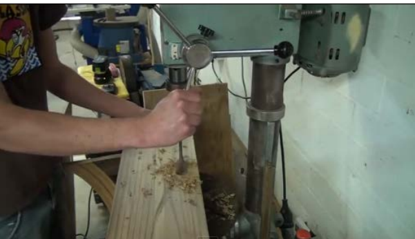
3. Drilling clearance hole on both rear & front vice jaws
