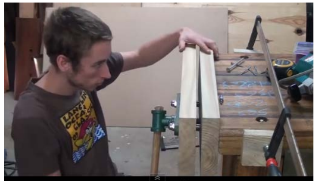
8. Checking final alignment & winding action
