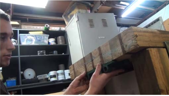
1. Lining up and screwing base to bench
