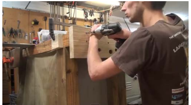
4. Screw rear vice Jaw in position
