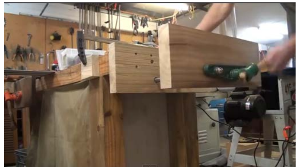
6. Line up front vice & wind tight in lock position
