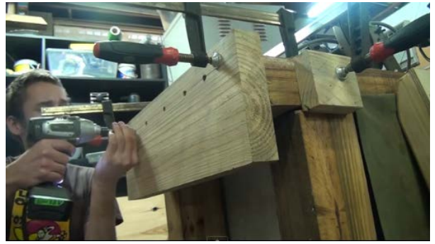
2. Temporary screw rear Jaw in position & mark holes
